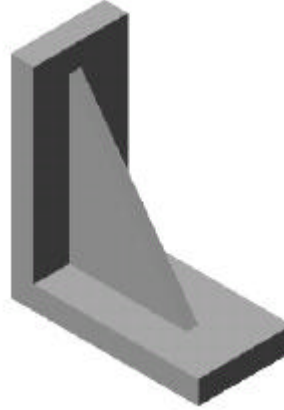
Rib applied selecting Parallel to sketch
